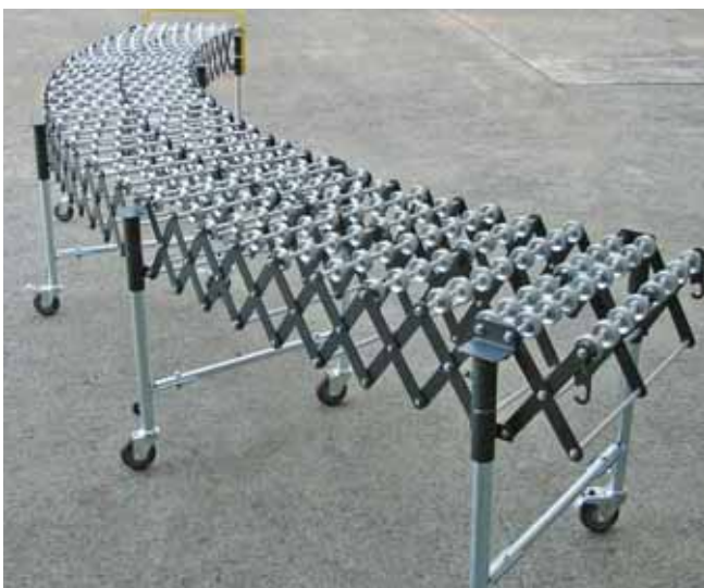
Steel skate and steel roller versions
