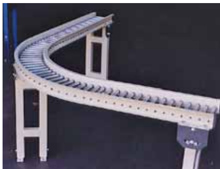
Special conveyor for small packages
