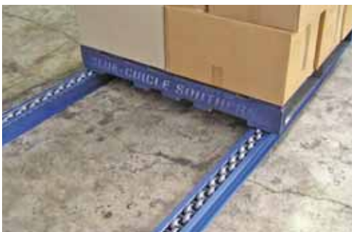
Wheel Track for Pallet Loads
